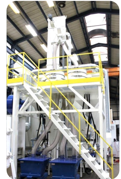
FIGURE: Bucket elevator with Airwash unit (left) & two media recycling system (right)
