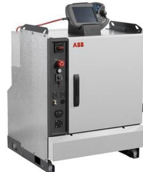
FIGURE: Robot Controller Unit (top) & Mobile HMI (left)
