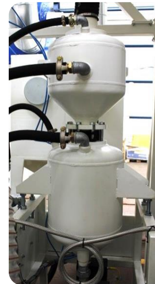
FIGURE: Double pressure vessel (left) & Magnavalves for nonferrous media (right)
