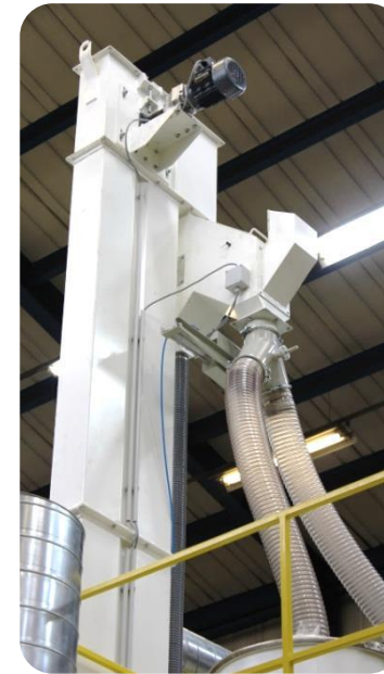
FIGURE: Bucket elevator with Airwash unit (left) & two media recycling system (right)
