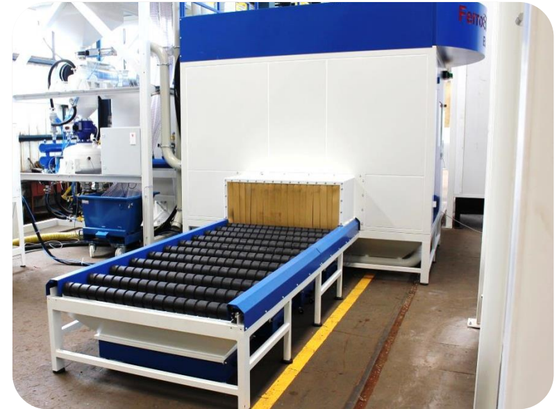
FIGURE: Heavy duty rubberized transport line
