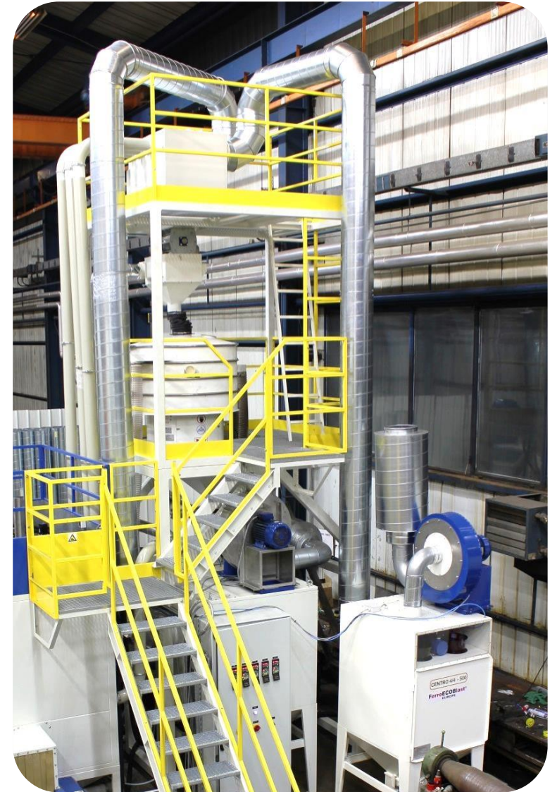
FIGURE: Pneumatic driven reclaim unit (above) & high capacity Sweco (left)
