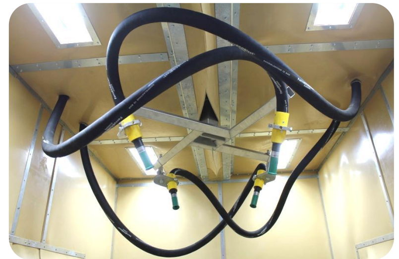
FIGURE: 1 axis Servo driven nozzle manipulator
