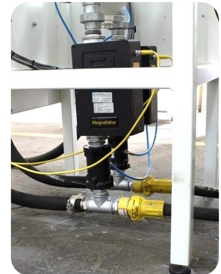
FIGURE: Double pressure vessel (left) & Magnavalves for nonferrous media (right)
