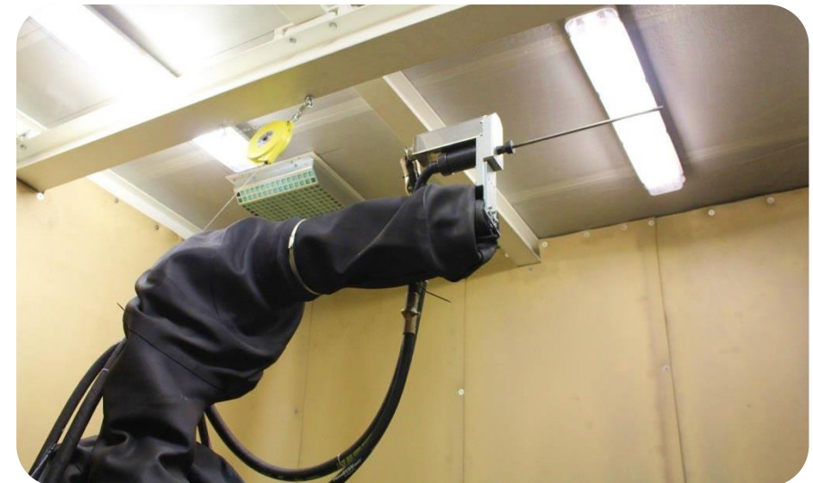
FIGURE: ABB Robotic industrial robot with rotating lance for smallest IDs (above) & Horizontal rotating lance assembly (left)
